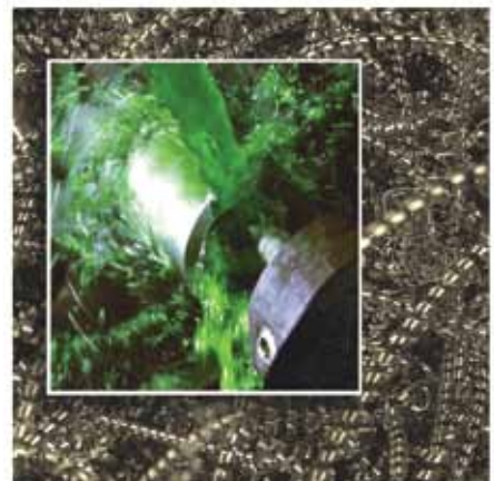
Steel chips: typical stringy, uncontrollable chip formation
