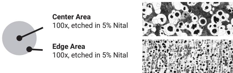
The microstructure consists of Types I & II nodular graphite as defined in ASTM A247. The matrix is ferrite with approximately 5-25% pearlite. The edge or rim will have a higher nodular count and will be mostly ferrite. Chill carbides will be less than 5% in any field at 100x and will be well dispersed.
