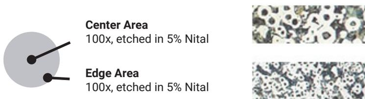
The microstructure consists of Types I & II nodular graphite as defined in ASTM A247. The matrix is ferrite with approximately 10-50% pearlite. The edge or rim will have a higher nodular count and will be mostly ferrite. Chill carbides will be less than 5% in any field at 100x and will be well dispersed.
